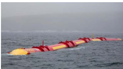
Figure 8: Pelamis wave power device [18].
